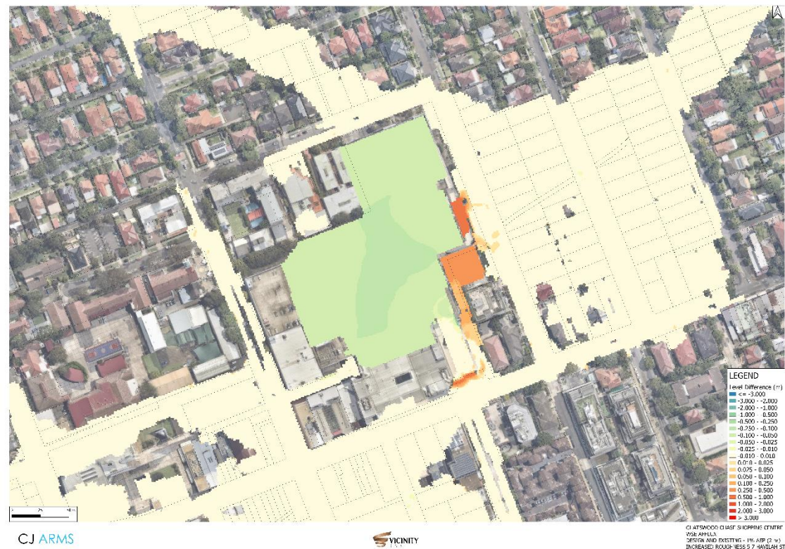
Figure 7: 1% AEP 2hr Design WSE Afflux with increased roughness in 5-7 Havilah Street carpark to simulate a potential blockage
