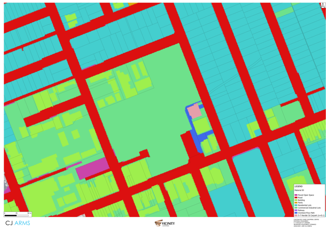
Figure 6: Material Roughness plot showing OFP (n=0.02) and 5-7 Havilah St Carpark (n=0.1)
